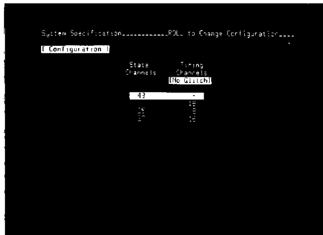
Figure 3-2. Default System Configuration For 1630D (1630A has 8 less channels)
